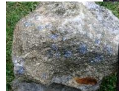
Visual molybdenum mined from the first bench Of the Kingsgate trial pit
