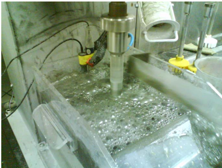
Flotation of sulphides from Khartoum greisen tin mineralisation
