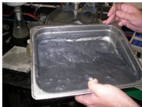
Bench scale metallurgical flotation testwork at AMMTEC laboratories in Perth. The molybdenite readily floats producing a high purity concentrate.
