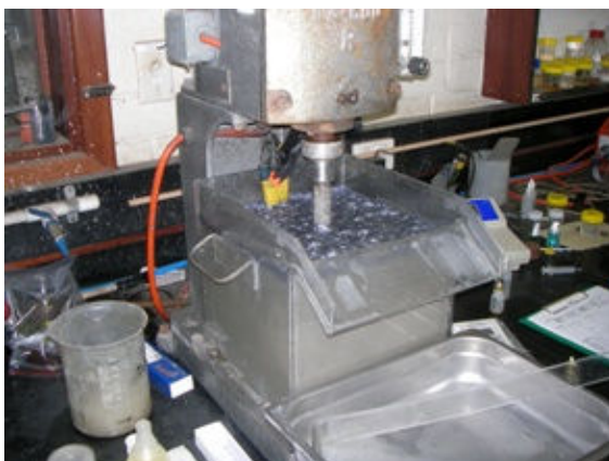
Bench scale metallurgical flotation testwork at AMMTEC laboratories in Perth. The molybdenite readily floats producing a high purity concentrate.
