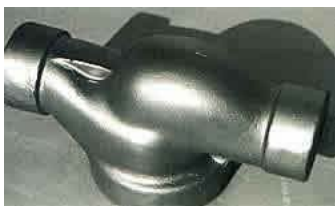
Valve casting containing up to 20% Mo to withstand severe corrosion and high temperatures (Source – IMOA)
